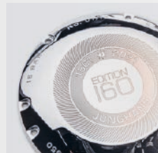
The edition logo engraved using a UKP laser onto a PT950 platinum case back.
