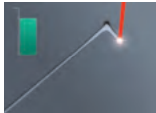
Untidy edges without in-line tailoring of laser parameters.
