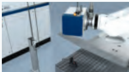
Positioning the programmable focusing optics above the sensor.
