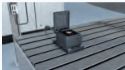
Focus sensor for positioning the laser beam on the workpiece.
