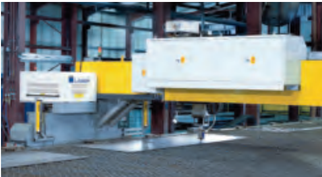
The stable resonator can even be installed on moving gantries.
