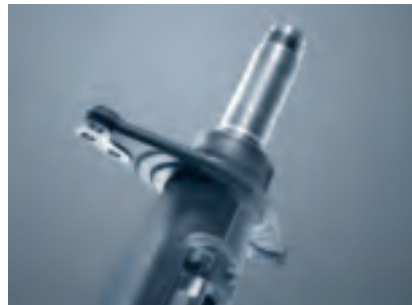
A truck axle welded with a CO 2 laser.
