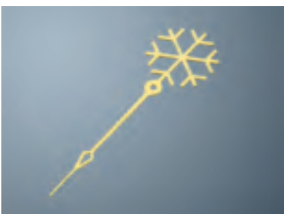
A watch hand cut with precision – as a result of real-time power control.
