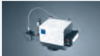
Mounted on the PFO, the pyrometer measures the temperature at the surface of the weld seam.
