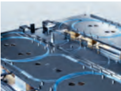
Optical arrangement in a TruFiber fiber laser.
