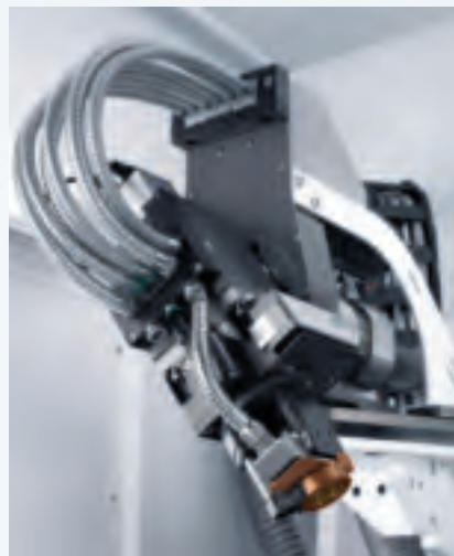
BEO D70 processing optics with motorized swivel mount on a robot.
