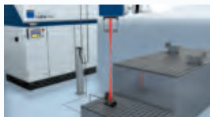
CalibrationLine measures the output power and makes adjustments where necessary.
