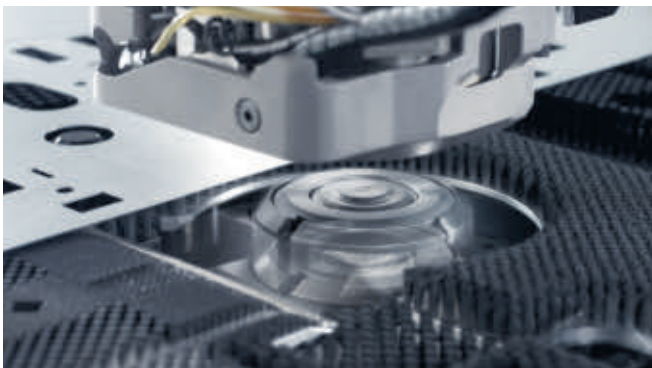
The active die provides for active reshaping from below and enables scratch-free processing.
